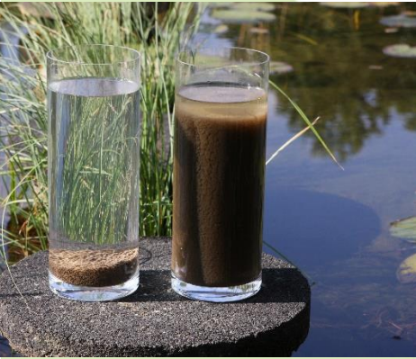
1 Granules form in the Nereda purification process
